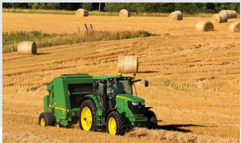
**Available on the 6170R, 6190R, and 6210R Tractors,** the optional 110- or 118-in axle also allows for group 47 duals, or John Deere exclusive group 48 duals in this horsepower segment.
